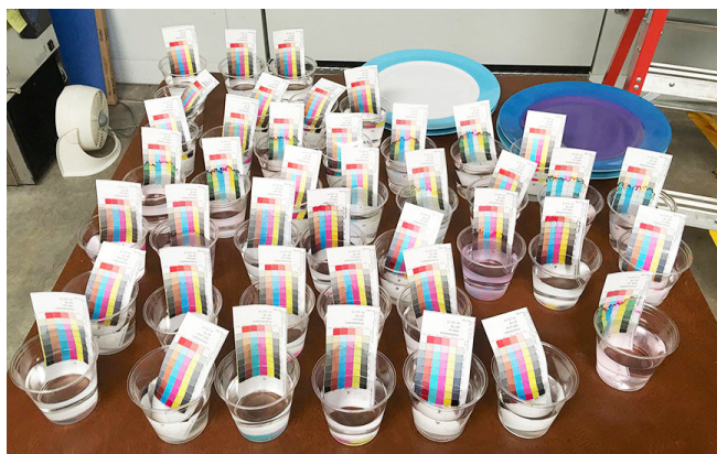
Figure 3. Test samples printed with pigment-based and dye-based inkjet inks undergoing the 24-hour “edge immersion” water-resistance test specified in Sec. 6.5 of ISO 18935:2016(E). This test was originally designed for RC-base and other multi-layer-structure photo papers and, in terms of applicability to commonly encountered types of water damage, the test may not be well-suited for evaluating the water-resistance of inkjet-printed plain paper documents.
